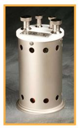
Model 9210A MI-Type standard has been developed through years of research by NRCC and Measurements International and is now offered as an improved resistor design to replace the L&N Thomas-Type One-Ohm Standard as well as other values. These improvements have been achieved through a new annealing process of the element and changes in the structural mounting. Historical data is now proving the Model 9210A to be the most stable oil filled resistor commercially available.
